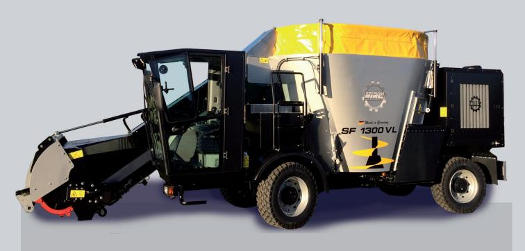
Mixing 1 or 2 vertical mixing augers with hydrostatic drive
