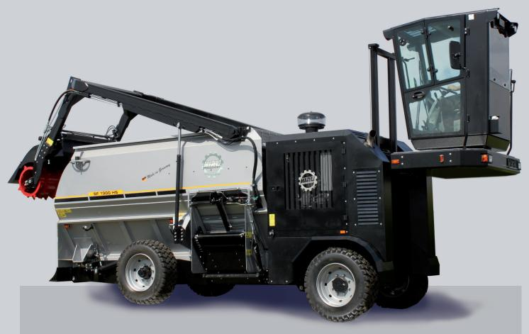
**Mixing** 3 horizontal mixing augers with hydrostatic drive
