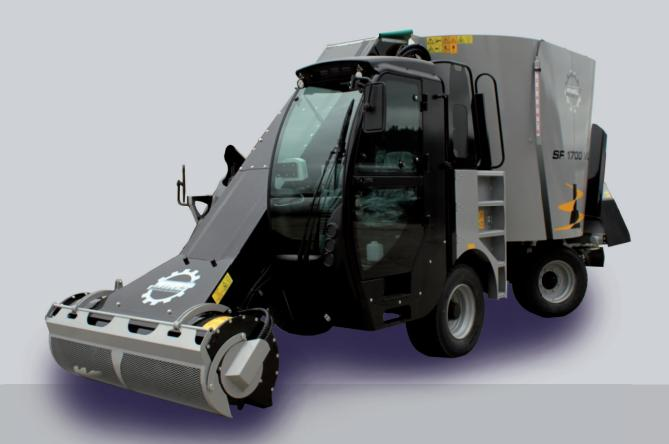
Mixing 1 or 2 verticale mixing augers with 2 speeds
