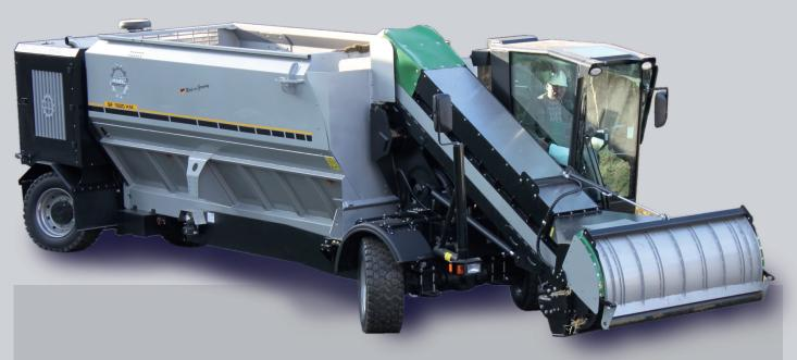
Mixing 3 horizontal mixing augers with hydrostatic drive
